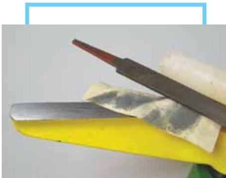
Use a file to smooth the nicks out of your toolrest. Sand the surface lightly and apply wax. Do this routinely and your turning will improve.
