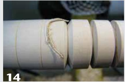
14 The circular chip that results from a V-groove cut.
