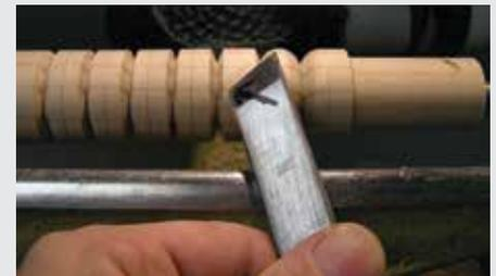
Plane a cylinder smooth with the skew, and mark out  $\frac{5}{8}$ " (16mm) intervals with a ruler and pencil or with dividers.
