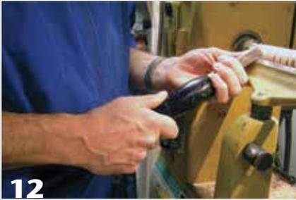
12 Present the skew with its long point down to form a V-groove, starting with the handle low, then lifting the handle to pivot the long point into the wood.
