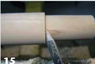
15 A paring cut is useful for facing off endgrain or cleaning up tenon shoulders.
