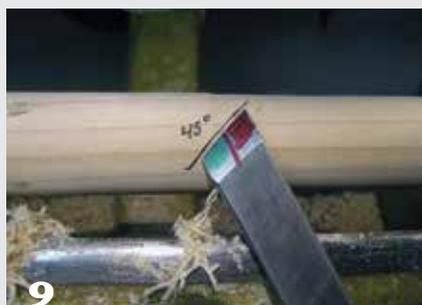
When making a planing cut, present the tool so the cutting edge is at a 45° angle to the blank. Keep the cutting action to the lower half of the edge, colored green.
