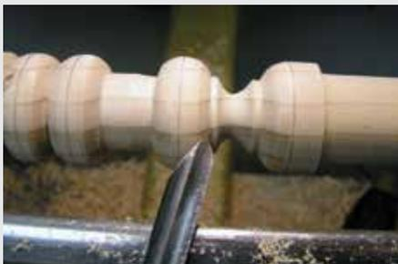
Start as you did in Exercise 2: plane a cylinder smooth with the skew, and mark out  $\frac{5}{8}$ " (16mm) intervals with a ruler and pencil or with dividers. Form V-grooves at every mark about  $\frac{1}{4}$ " (6mm) deep, then mark centerlines between all the V-grooves. After rolling beads as you did in Exercise 2, turn away every other bead using a peeling cut.
