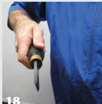
Consider how your hand must rotate when forming beads. For the right side of a bead, it rotates clockwise; for the left side, counterclockwise. In both cases, the finishing position is with the tool edge vertical and your hand as though you are going to shake hands with someone.
